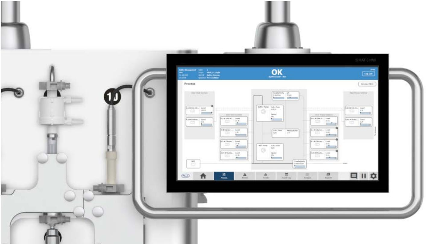
Fig 11. Touchscreen HMI with on-screen visual instructions.
