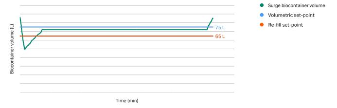
Fig 9. In-line buffer dilution level control in process biocontainer at a draw rate of 1200 L/h and 10-fold dilution factor.
