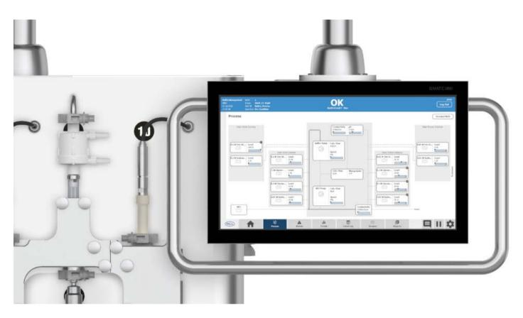
Fig 11. Touchscreen HMI with on-screen visual instructions.
