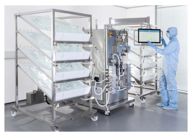
Fig 3. Touchscreen, maneuverable human machine interface (HMI) for efficient operator interaction.
