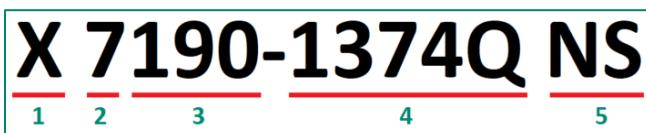
1. Prototype - an 'X' prefix indicates that the drawing is a prototype.
