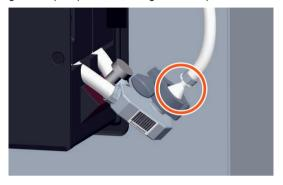
10 Connect the other end of the jumper tubing to the right side of the pump tubing on the isocratic pump (**P-201**).
