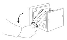
Take the pump tubing and the jumper tubing out of the gradient flow section package.
