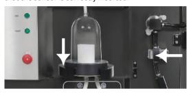
3 Temporarily hang the outlet manifold on the cabinet door.
