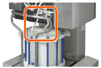
6 Turn the installation switch to the **COLUMN INSTALL** position.
