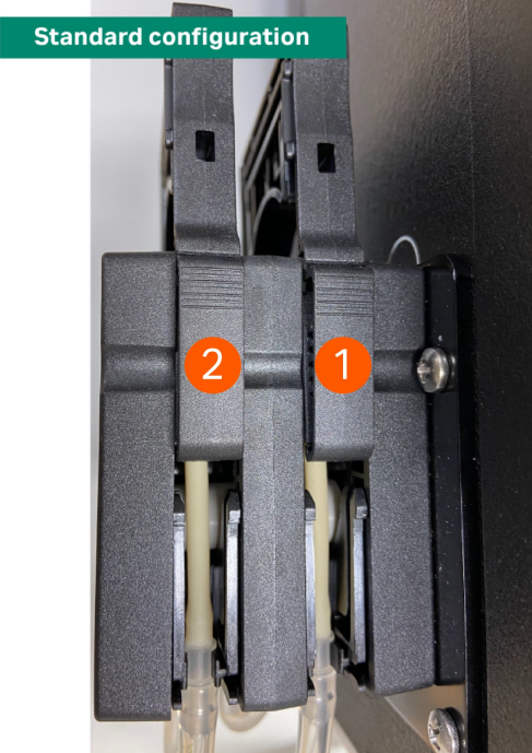
Peristaltic pump 2 mm ID tubing connected to both position 1 and position 2.
