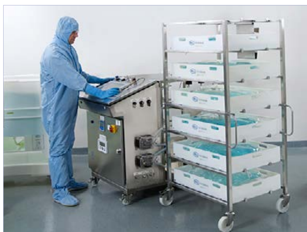
Figure 6 Single-use virus filtration system operation
