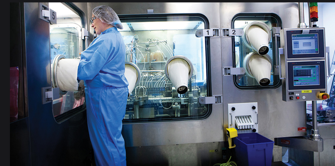
A conventional filling system with glove ports
