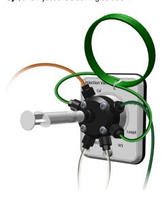
5 Fill a syringe with distilled water. Connect the syringe to injection valve port **Syr**, and inject the distilled water.
