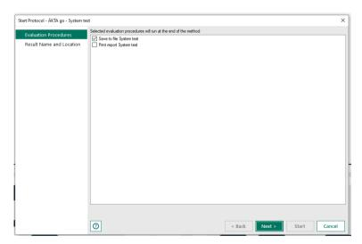
5 Specify the details of the result file from the performance test. Click **Start** to start the performance test.
