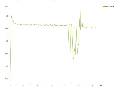
9 If the pressure does not stabilize within a few minutes, repeat the procedures to prime the inlet tubing and purge the pump. If the pressure still does not stabilize, refer to the ÄKTA go User Manual for further instructions.
