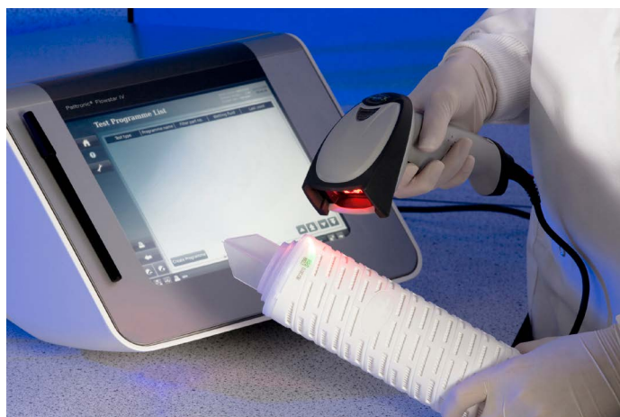
Fig 2. Emflon HTPFR cartridge being scanned with a Palltronic® barcode reader and connected to a Palltronic Flowstar IV integrity test instrument.
