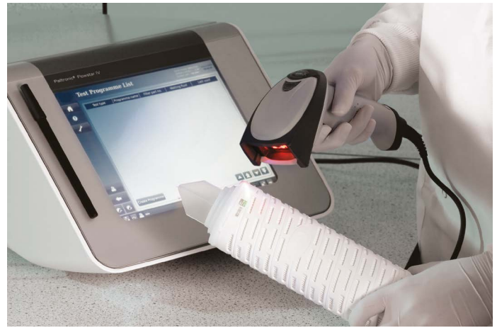
Fig 7. Scanning a barcode on a Pegasus SV4 virus removal filter cartridge using a Palltronic barcode reader and Palltronic Flowstar IV filter integrity test instrument.
