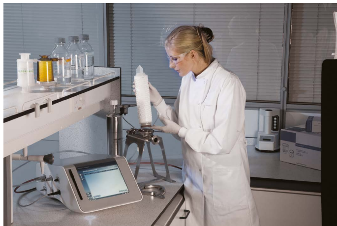
Fig 5. Integrity testing Pegasus SV4 virus removal filter cartridges with a Palltronic® Flowstar filter integrity test instrument.
