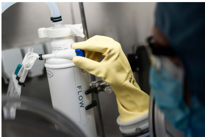
Fig 2. Venting a Kleenpak Spectrum capsule on an automated filtration system.
