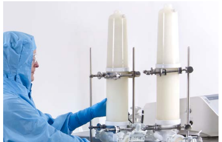
Fig 4. Kleenpak Presto sterile connector attached to filter cartridges.
