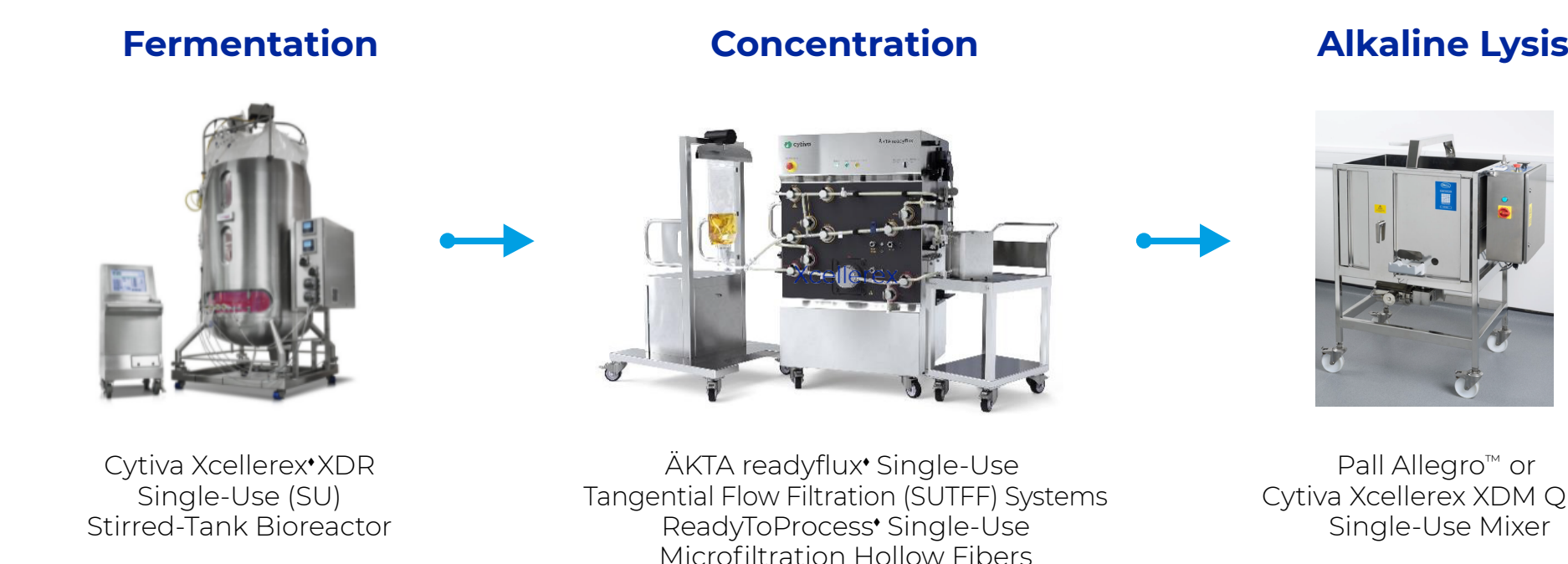
Figure 2 Plasmid DNA downstream process
