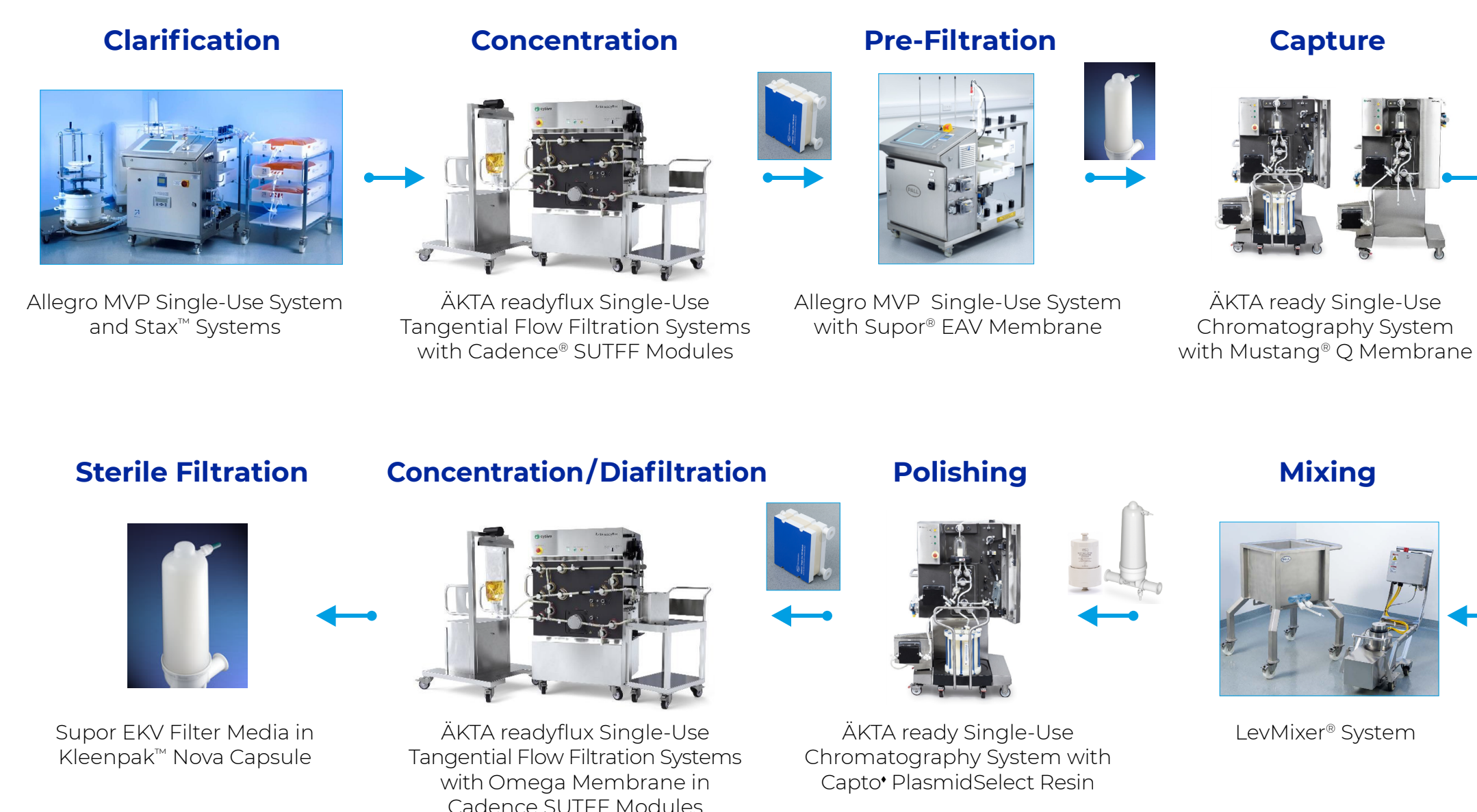
Figure 2 Plasmid DNA downstream process
