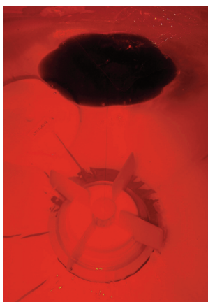
Figure 1 Solution homogeneity in the biocontainer during mixing
