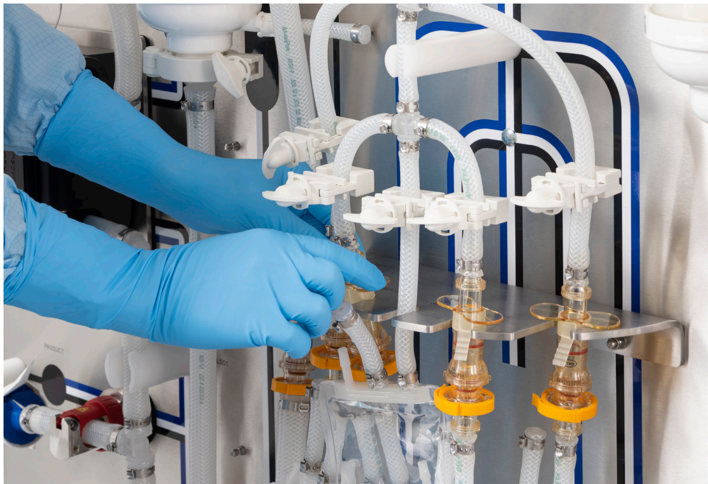
Fig 25. Shadow board visibly guides the user and reduces installation errors.
