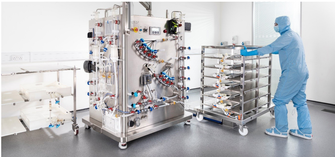
Fig 7. Installing an all-in-one biocontainer bag system on the weighing platform.
