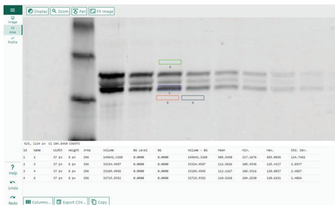
**Fig 7.** Area analysis in ImageQuant™ TL includes analysis of region of interest and background. The area is measured in units of pixels (width times height). After background subtraction, the mean pixel intensity is compared to the background and the background noise level.
