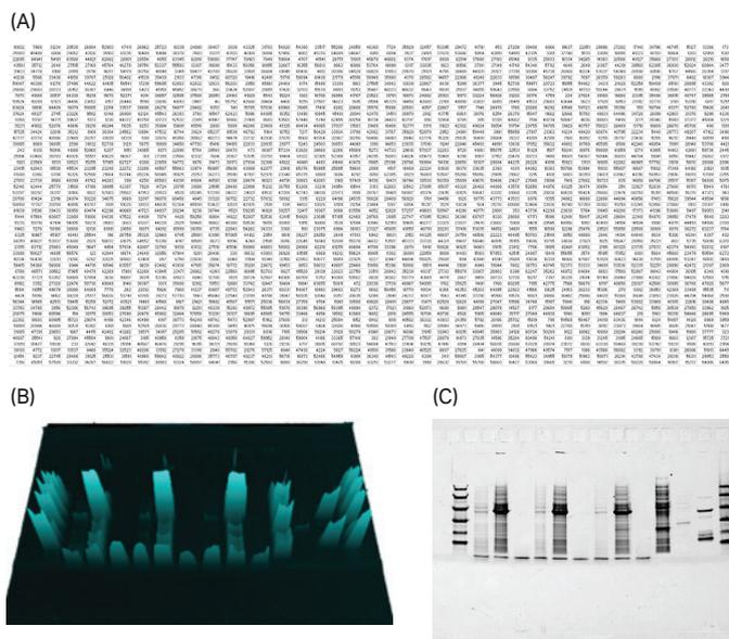
**Fig 2.** An image is a matrix with intensity values (A) which can be visualized in three (B) or two (C) dimensions. Each matrix element corresponds to a physical pixel on the detector. The intensity values are mapped to a gray or a color-scale to view the three-dimensional data in a 2D image. The screenshots were taken from ImageQuant™ TL analysis software.
