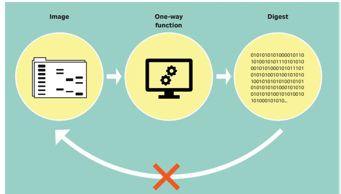
**Fig 8.** One-way secure hash algorithms compute a fixed-length message digest from arbitrary length data. An input of varying length is used to create the output, however, the output cannot be used to de-construct the input.
