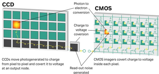
**Fig 1.** The two most common types of camera detectors, charge-couple device (CCD) and complementary metal-oxide semiconductor (CMOS).
