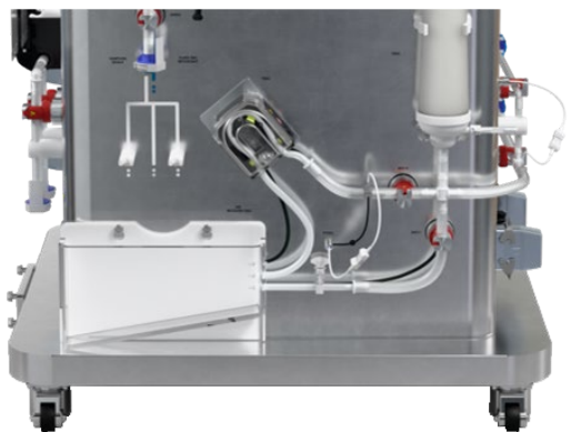
Fig 2. Recovery pump and bag for enhanced product recovery located on the drug product filtration system.
