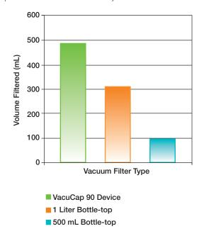
VacuCap 90 (0.2 μm) filter device performance as compared to that of competitive vacuum filter units with 0.2 μm Cellulose Acetate membrane. Filtration conducted at 21 °C (70 °F) and 38 cm Hg (15 in. Hg) vacuum. Volumes reflect a filtration time of five minutes.
