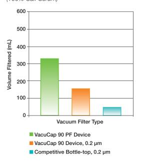
Filtration conducted at 21 °C (70 °F), 50 cm Hg (20 in. Hg) vacuum, five minute filtration time. Actual results may vary depending upon type and concentration of serum, liquid temperature, and applied vacuum.
