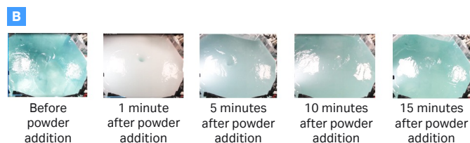
Fig 5. NaCl 1.5 M mixing in the Xcellerex magnetic mixer 3000 L.
