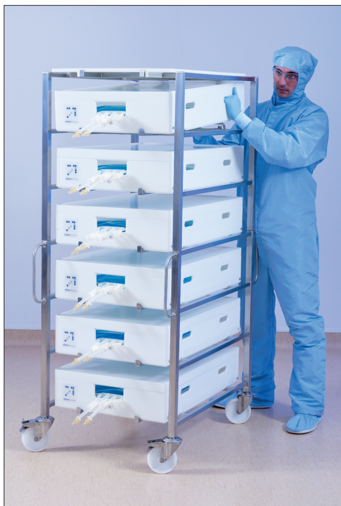
Single column bioprocessing workstation with 20 L Allegro trays and systems
