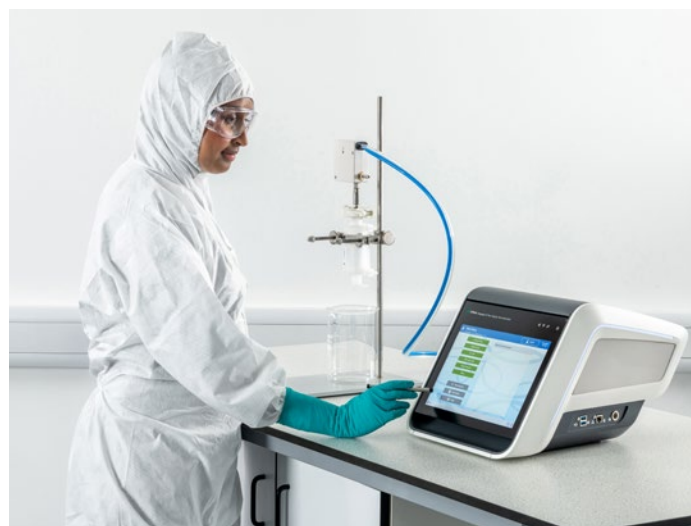
Fig 2. Integrity testing a filter capsule.
