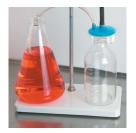
Connect the vacuum tubing to the port marked "VACUUM" on the VacuCap device. Refer to product insert for safety precautions.
