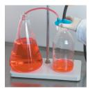
While holding the VacuCap device securely on the filtrate container, start the vacuum. The VacuCap device will seal securely to the container top and fluid will be drawn.
