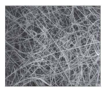
Tissuquartz Filters – High temperature use for analysis of acidic gases and stack sampling aerosols. Ultra-pure soft water processing reduces residual ion content.
