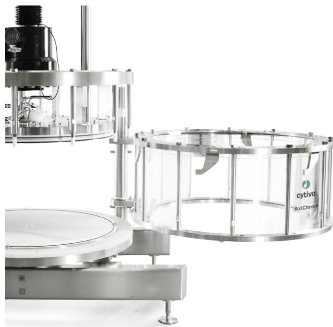
Fig 8. AxiChrom column in swing-out mode provides easy access to bed supports and O-rings. In multipurpose facilities, changing plastic bed supports for a new campaign is quick and hassle free.
