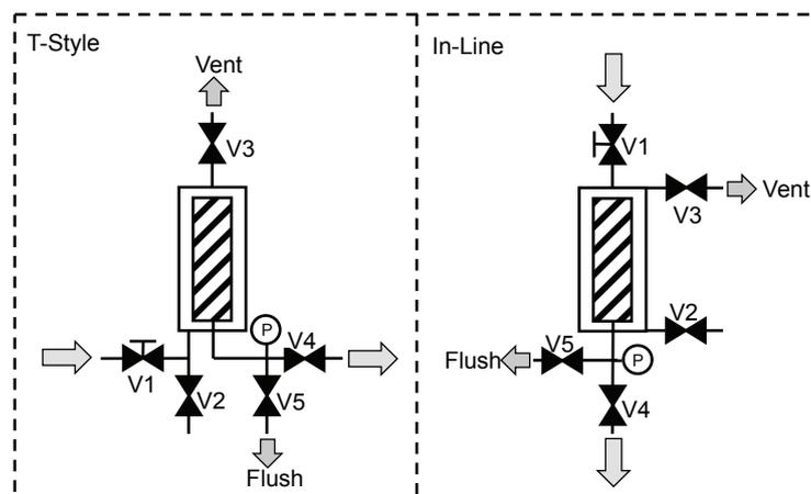
The filter can be wetted by filling from the inlet (V1) and vented over the vent valve (V3) of the housing (or an additional vent introduced at the top of the filter) while keeping the valve on the downstream side of the housing closed. Slow filling can either be achieved by throttling V1 or by using a pump at low speed. The downstream valves V4 and V5 remains closed during filling.
