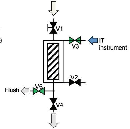
**Note:** If neither V4 or V5 can be opened or if a non-vented bag is connected to the open valve the pressure downstream must be monitored especially in the initial phase of the pressurization by the integrity test instrument in order to become aware of pressure increase due to insufficient wetting or major leaks in the membrane for example.
