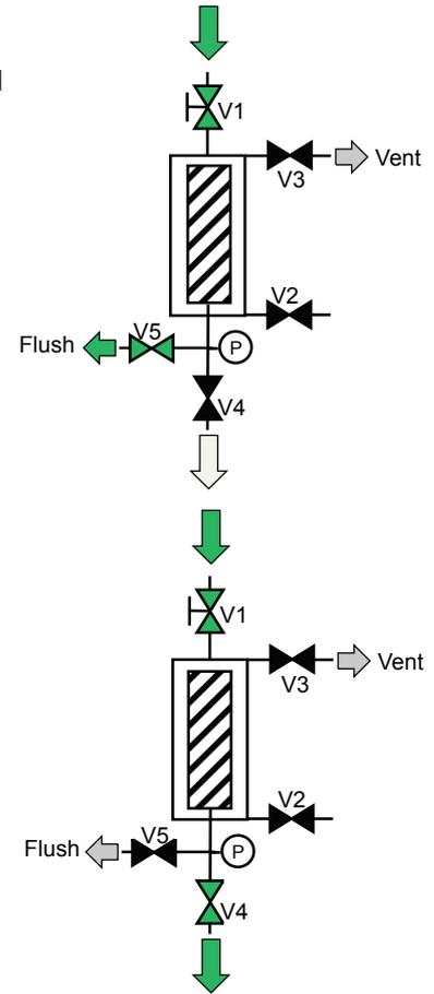
3. Open valve V4 to start filtration (V3 is closed at this point)
