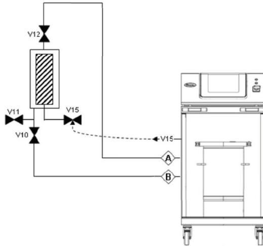
The valve downstream of the filter is essential as during the filling and the soaking phase of the wetting cycle the water must be kept in the housing.
