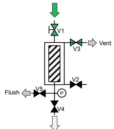
2. If dilution of the product by the remaining wetting fluid in the membrane should be avoided or further flushing is required to remove extractables/leachables, the vent valve V3 should be closed and V5 should be opened for the appropriate flushing.
