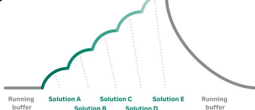
Fig 5. **Poly** command injects 3 to 5 different solutions in sequence with no time delay or liquid between in the order Solution A to E.
