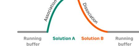
Fig 3. **Dual** command injects two different solutions in sequence with no time delay or liquid between in the order Solution A and Solution B.
