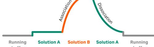
Fig 4. **ABA** command injects two different solutions in sequence with no time delay or liquid between in the order Solution A, Solution B, then Solution A.
