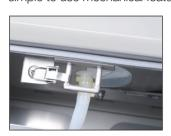
Bottom outlet port securely clamped and clamps locked into place ensuring no possible lateral or up and down movement of the portbiocontainer joint
