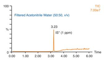
Detection - Mass Spec: ES+ Mode; Mass Range: 100.00-1400.0 Column: Waters Acquity◆ UPLC BEH 1.7 µm - 2.1 x 50 mm
