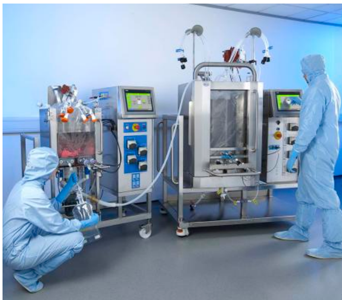
Setting up a transfer from an Allegro STR 50 L bioreactor to an Allegro STR 200 L bioreactor
