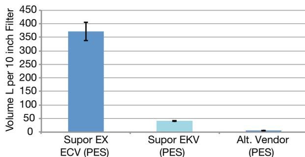
The throughput performance of Supor EX grade ECV filters with HA solutions is attributable to a unique membrane layer combination incorporating a highly asymmetric upstream membrane layer. This high performance is augmented in a 10-inch filter device (Figure 3) owing to a laid over pleat membrane geometry and cartridge design which enables a high filtration area per 10-inch filter element, in excess of 1 m<sup>2</sup>.
