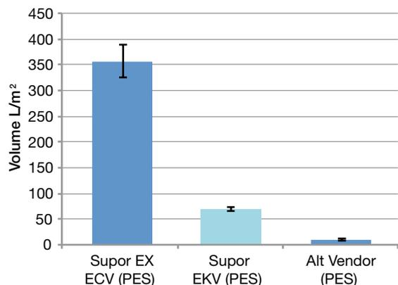
**Figure 3***Predicted 10-inch filter cartridge throughput performance with 1.8 MDa Hylauronic Acid, assuming linear scale-up for all filters*
