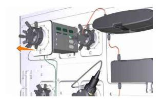
4 Disconnect the cable and secure it in the slit.
