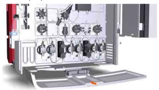
6 Unscrew the three screws holding the hinge to the pump cover and remove the hinge.
