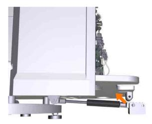
9 Put the outer shaft back into place, and screw the two countersinked screws back.
