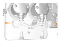
7 Unscrew the lower check valve using an adjustable wrench.
