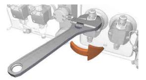
6 Unscrew the two white plastic screws located below each pump head. Pull the plastic connectors to the sides to release the inlet manifold.
