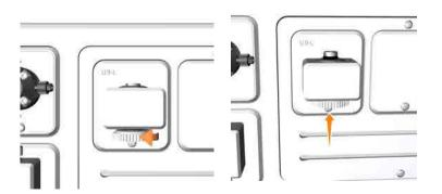
4 Pull the flow cell upwards out of the monitor. Hold the flow cell by the top part with the O-ring: do not touch the optical surfaces of the flow cell.
