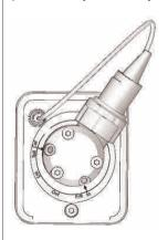
Valve which enables the pH electrode to be included in the flow path or by-passed during a run. The pH electrode may be calibrated when installed in the pH Valve. It also enables the flow restrictor to be included in the flow path (default position) or by-passed during a run.
