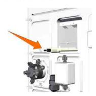
6 Connect the cable to the module to be installed.
