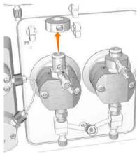
5 Unscrew the plastic nut of the upper check valve using an adjustable wrench, and gently lift off the upper check valve.
