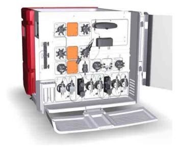
The Extension box can be used to hold modules connected to the back of the instrument. See Section 2.6.3 Extension box, on page 52 for more information.
