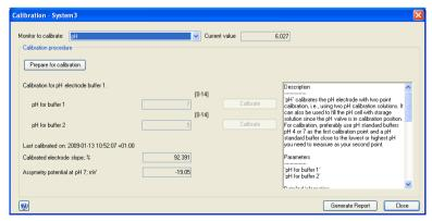
2 Set the pH monitor as the monitor to calibrate by clicking **pH** on the **Monitor to calibrate** menu.
