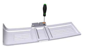
7 Screw the three screws back to the pump cover and put the pump cover in a safe place.
