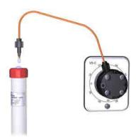
7 Connect a piece of tubing to the bottom of the column.
