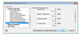
3 Enter new values in the **Detector-Frac**, **Detector-Outet valve**, **Restrictor volume**, and **pH cell volume** fields if necessary
