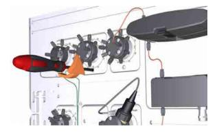
3 Remove the valve module.
