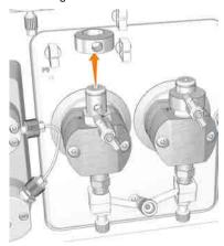
3 Unscrew the plastic nut of the upper check valve using an adjustable wrench, and gently lift off the upper check valve.
