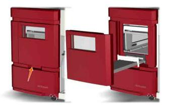
Place the rack on the tray support of the fraction collector drawer. Make sure that the front of the rack (marked with the Cytiva monogram) faces the front of the drawer and is hooked onto the two pins.
