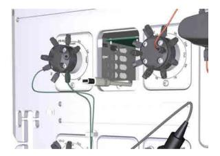
5 Connect the cable to the new valve module.
