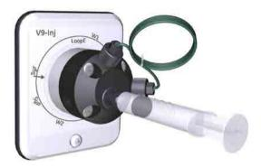
6 Fill a syringe with distilled water. Connect the syringe to Injection valve port **Syr**, and inject the distilled water.
