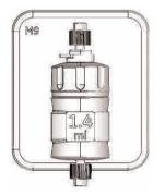
Mixes the buffers delivered from the system pumps to a homogeneous buffer composition.
