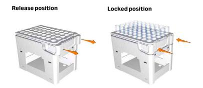
2 After fractionation, pull the QuickRelease device to the release position and remove the tubes containing the fractions you want.
