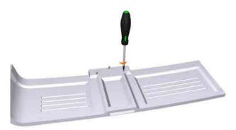
8 Put the inner shaft back through the hinge and damper, and push the hinge into place.
