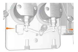
8 Unscrew the lower check valve using an adjustable wrench.
