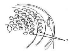
Push the flexible bowl out at each rib and snap the tube holder under the top lip of the rib (8).
