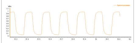
Incident: Inlet check valve is loose.
