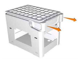
Place the tubes and deep well plates in the cassettes. Make sure that the deep well plates are rotated so that the well marked A1 is positioned above the A1 marking on the cassette.
