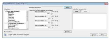
Select Pumps and pressures →System flow and set Flow rate to 0.01 ml/min.
