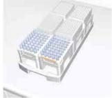
5 Open the fraction collector drawer by pressing the handle upwards, and pulling out the drawer.
