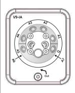
Inlet valve for System Pump A with seven inlet ports and integrated air sensor.
