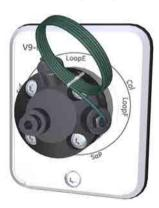
4 Connect tubing to Injection valve port W1, and direct this tubing to a waste container.
