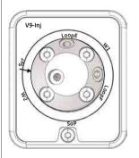
Valve which directs sample onto the column. For further information, refer to Section 3.5 Injection valve, on page 67.
