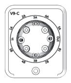
Column valve which connects up to five columns to the instrument, and directs the flow to one column at a time. The column valve features two integrated pressure sensors.
