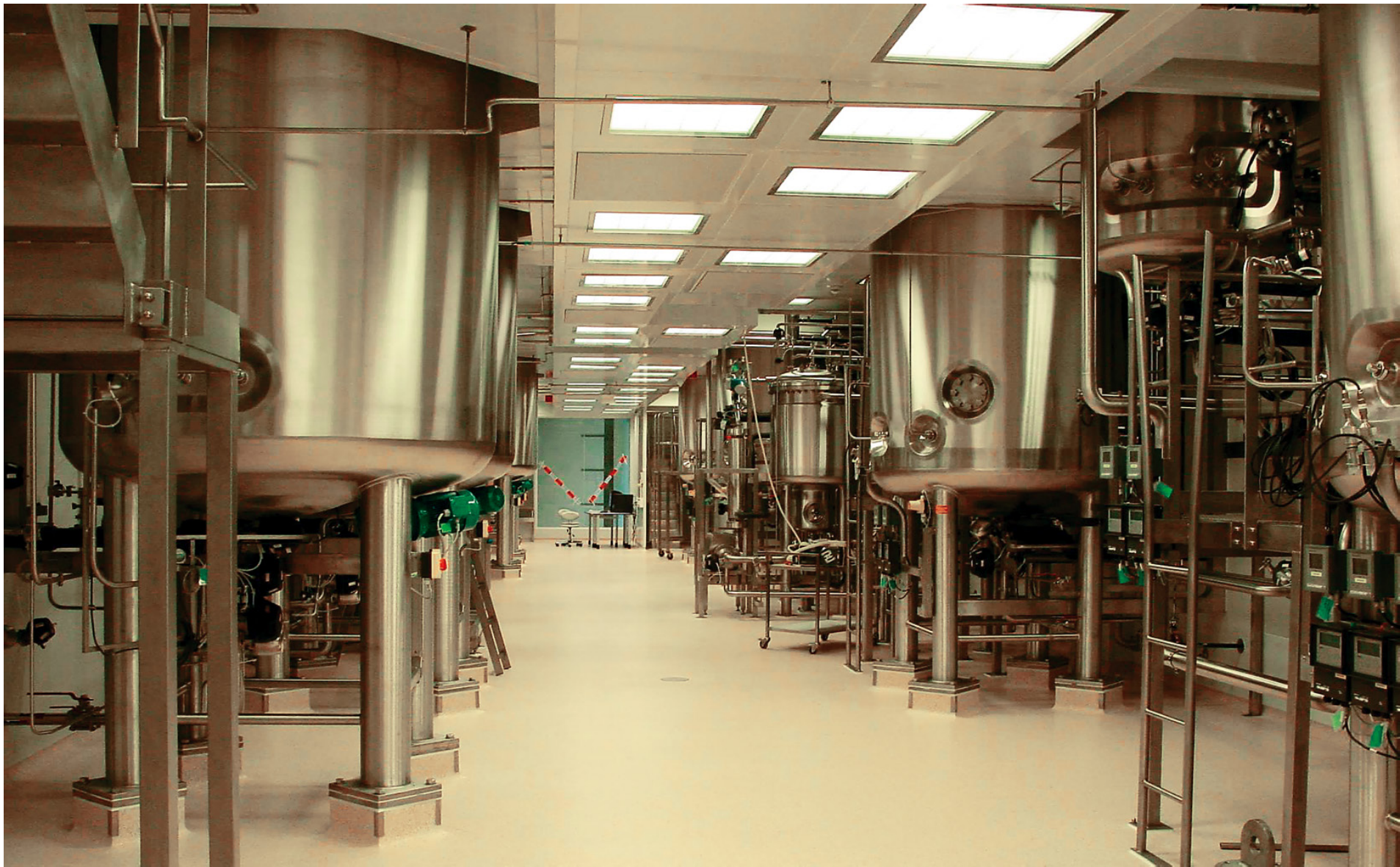
Fig 2. Influenza production plant (6000 liter vessel for cultivating Vero cells on Cytodex™). Courtesy of Baxter Biosciences.
