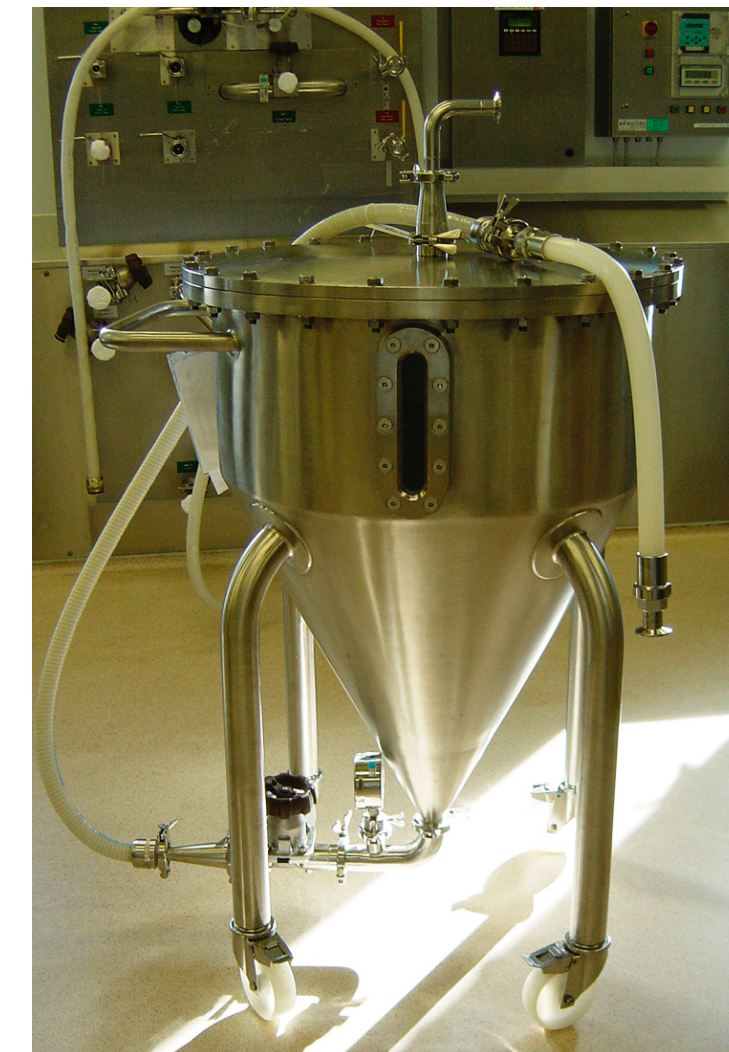
Fig 83. A fluidized bed for Cytodex cell separation. Courtesy of Wertheim Chemie, Switzerland.
