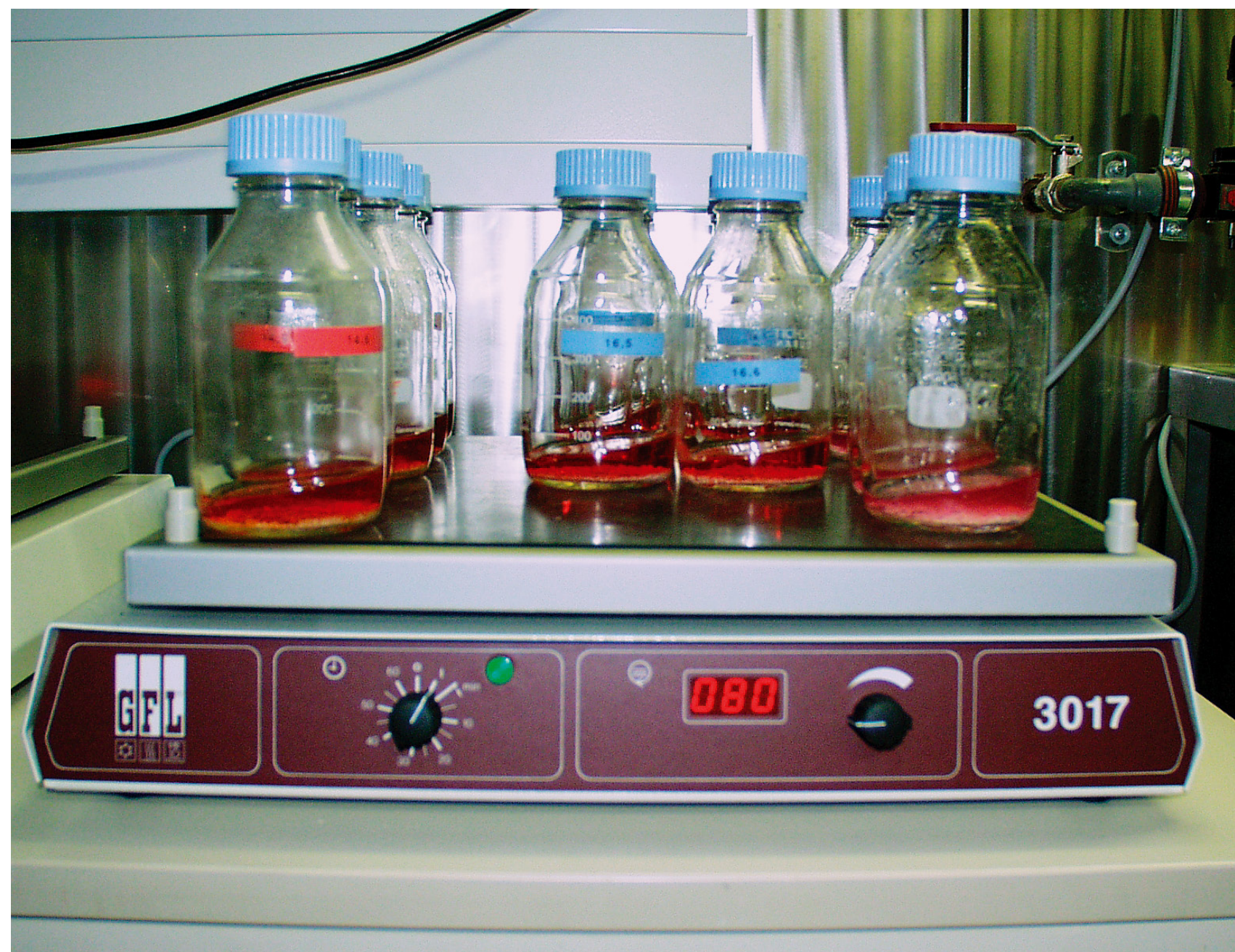
Fig 45. Small-scale macroporous microcarrier test configuration (a). Large bottles (e.g., 450 cm 2 roller bottles) on an orbital shaker (b).
