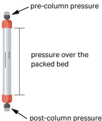
**Fig 3.** Pre-column and post-column measurements.
