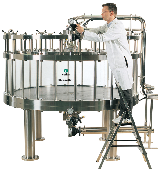
Fig 1. A Chromaflow column, 2000 mm i.d.
