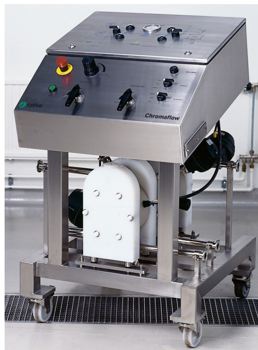
Fig 5. Chromaflow Packing station Pack 100.
