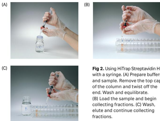
**Fig 2.** Using HiTrap Streptavidin HP with a syringe. (A) Prepare buffers and sample. Remove the top cap of the column and twist off the end. Wash and equilibrate. (B) Load the sample and begin collecting fractions. (C) Wash, elute and continue collecting fractions.
