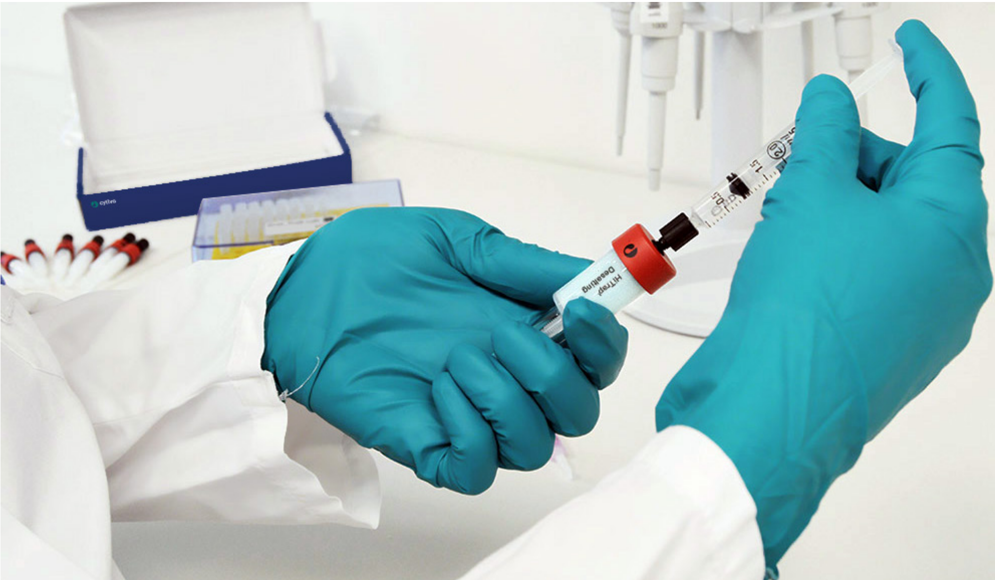
Fig 5.8. HiTrap Desalting column operated by syringe.
