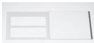
Figure 3.3: Open the gel cassette with the hinge downward.
