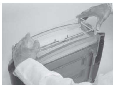
Figure 3.15: Seat the upper buffer chamber.
