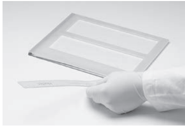
Figure 3.11: Push the strip into place.
