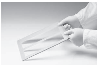
Figure 3.9: Snap the cassette shut.
