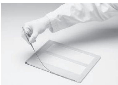
Figure 3.10: Place the IPG strip onto the glass lip.
