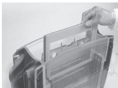
Figure 3.14: Insert the cassettes into the cassettes carrier.
