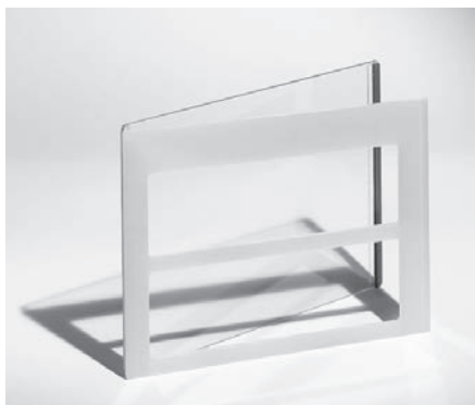
Figure 2.1: Precast Gel Cassette holds the gel vertically.
