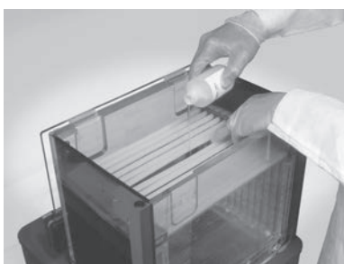
Figure 3.1: Add the anode buffer.
