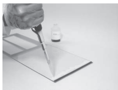
Figure 3.4: Pipette a line of gel buffer onto the glass plate.
