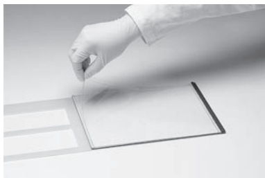
Figure 3.6: Lower the gel onto the glass plate.
