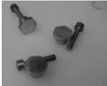
Fig 2-34. Bolts and fittings holding the liquid distributor in the lid.
