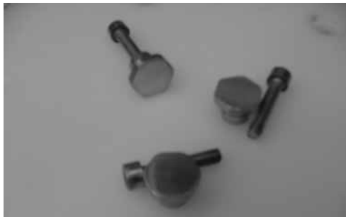
Fig 2-19. Bolts and fittings holding the liquid distributor in the lid.
