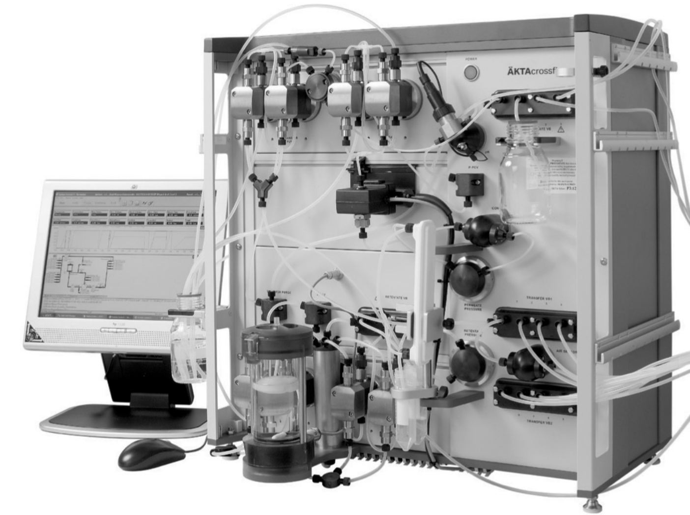
Fig 30. ÄKTAcrossflow has a compact and sanitary design.
