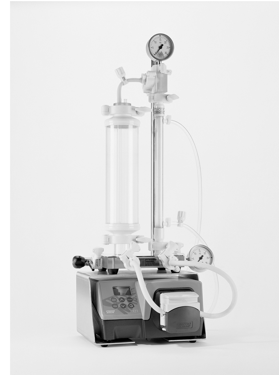
Fig 32. QuixStand laboratory scale separations system QSM-03SP with Xampler 4M cartridge, shown with 1-liter reservoir and PRP-09WM peristaltic pump
