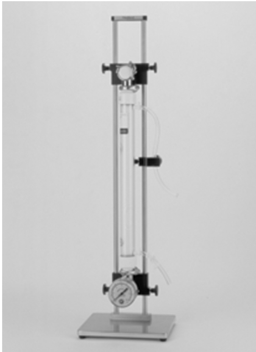
Fig 33. Standard FlexStand system FS-01S with size 9 cartridge installed
