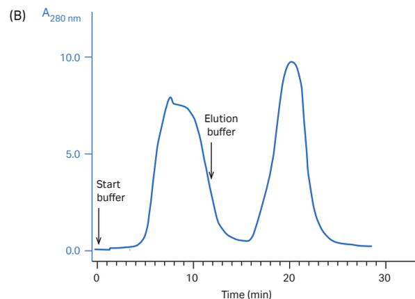
**Fig 4.** Scale-up from (A) a laboratory column (bed volume 80 mL) packed with SP Sepharose Fast Flow to (B) a column suitable for industrial production (bed volume 10.5 L) with retained packing and separation characteristics.
