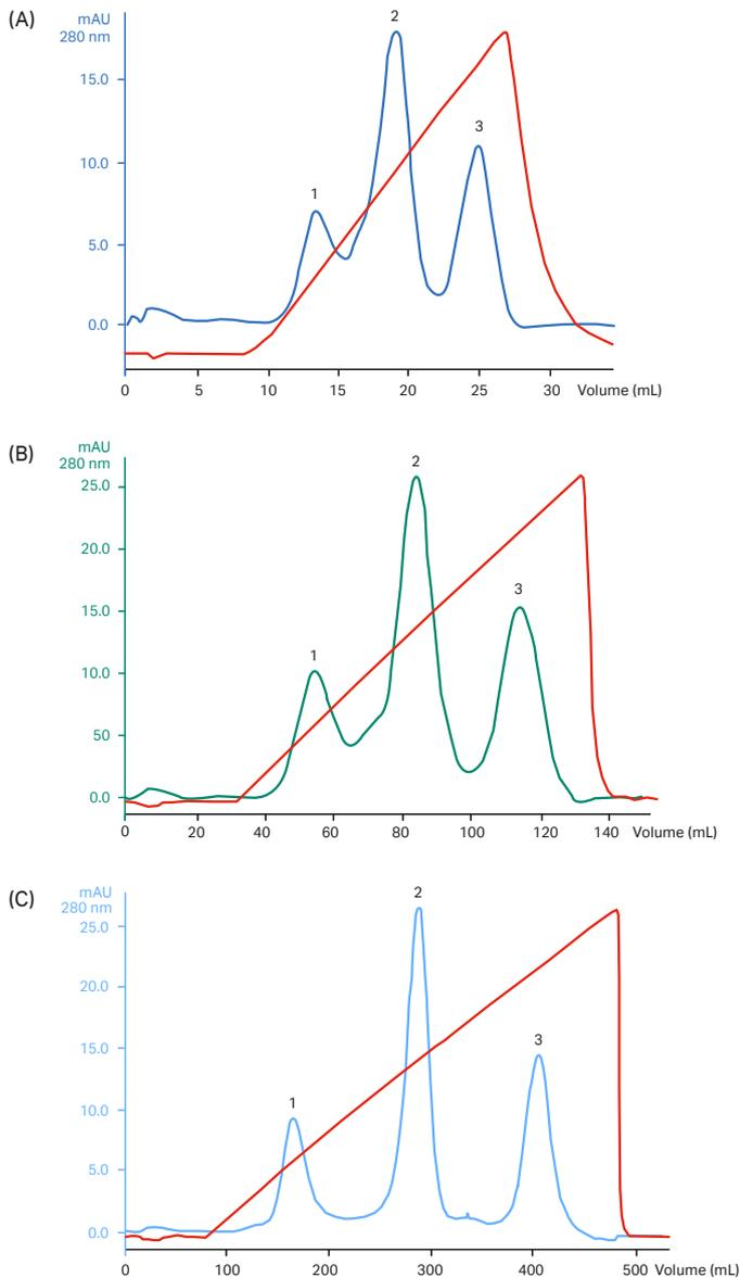
**Fig 3.** Five-fold and twenty-fold scale-up on prepacked Q Sepharose Fast Flow columns. (A) HiTrap Q FF, 1 mL ( $0.7 \times 2.5$  cm); (B) HiTrap Q FF, 5 mL ( $1.6 \times 2.5$  cm); (C) HiPrep Q FF 16/10, 20 mL ( $1.6 \times 10$  cm).
