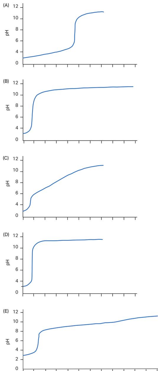
**Fig 2.** Titration curves showing the pH ranges over which the functional groups are charged. (A) CM Sepharose Fast Flow; (B) SP Sepharose Fast Flow; (C) DEAE Sepharose Fast Flow; (D) Q Sepharose Fast Flow; (E) ANX Sepharose 4 Fast Flow (high sub).
