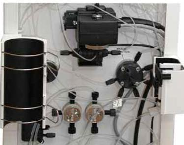
**CORRECT.** The large column holder correctly mounted.
