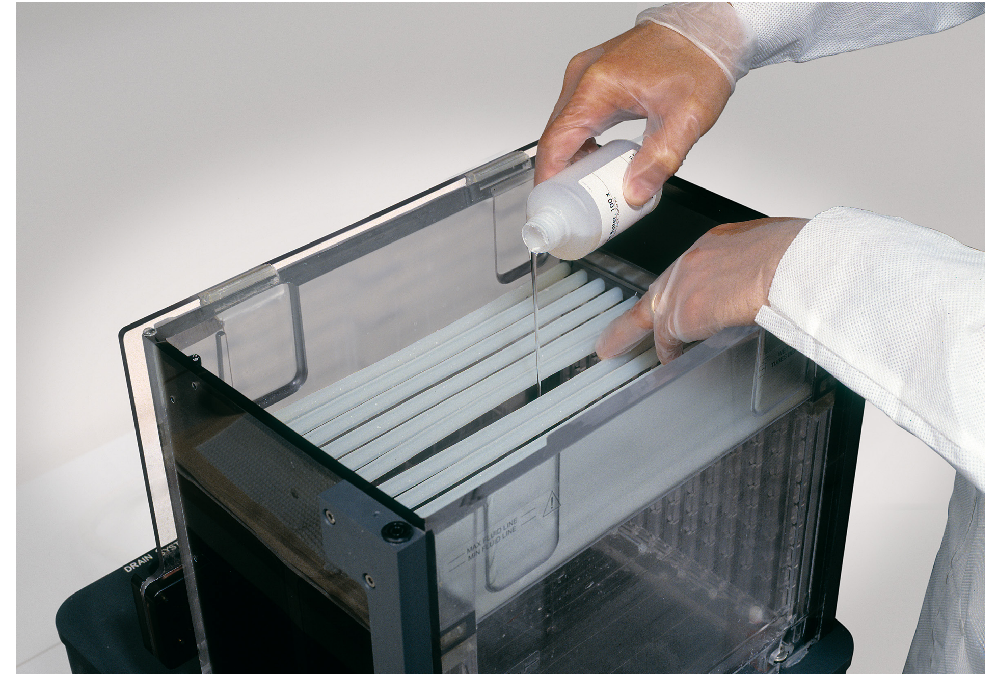
Fig 35. Spreading the tubing elements apart with one hand while pouring the solution with the other (to avoid pouring the 100× anode buffer onto the tubing).
