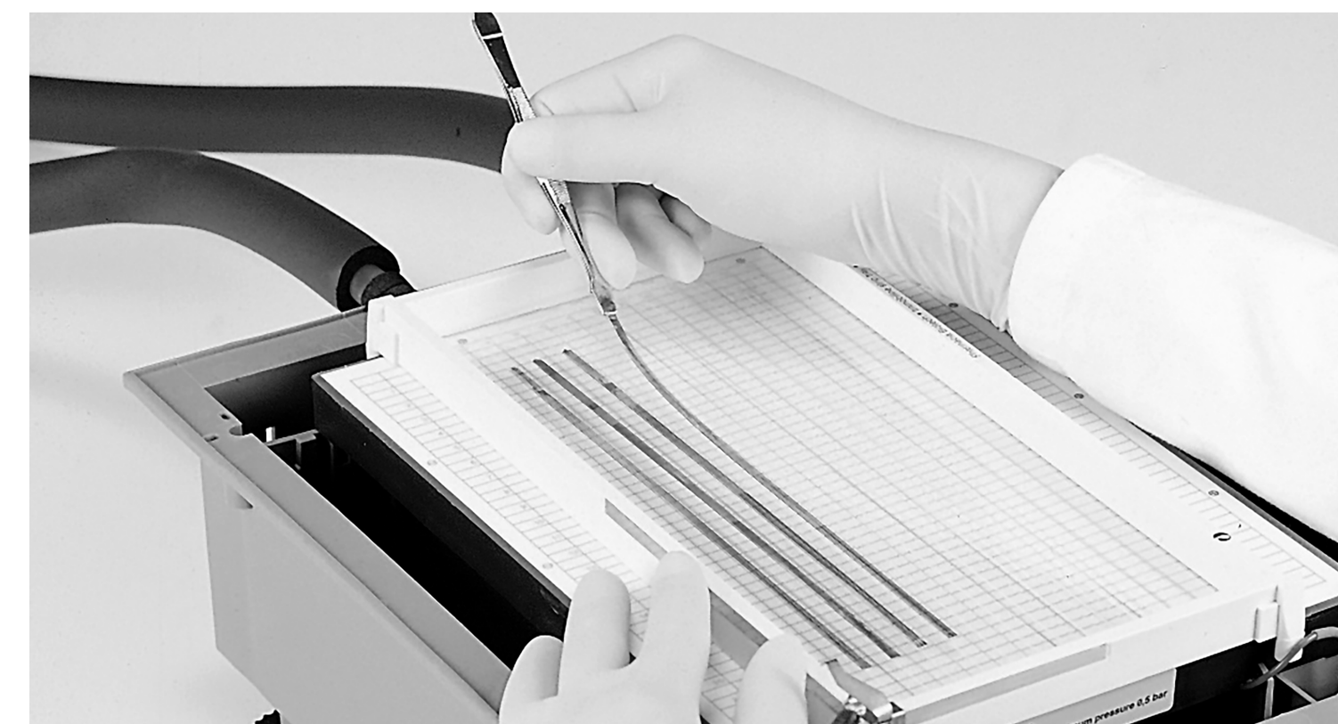
Fig 48. Positioning Immobiline DryStrip gels in the Immobiline DryStrip aligner.
