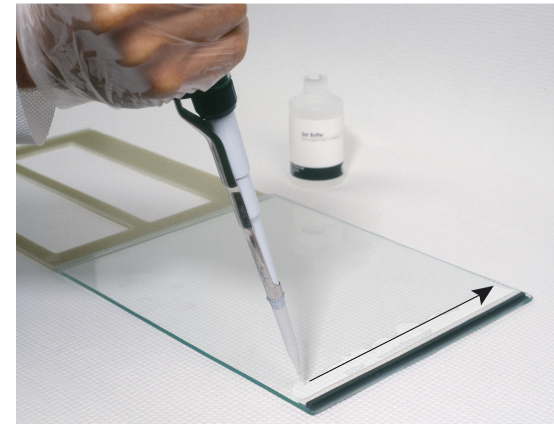
Fig 36. Pipetting a streak of gel buffer onto the glass plate. The arrow indicates the direction of motion in applying the streak.
