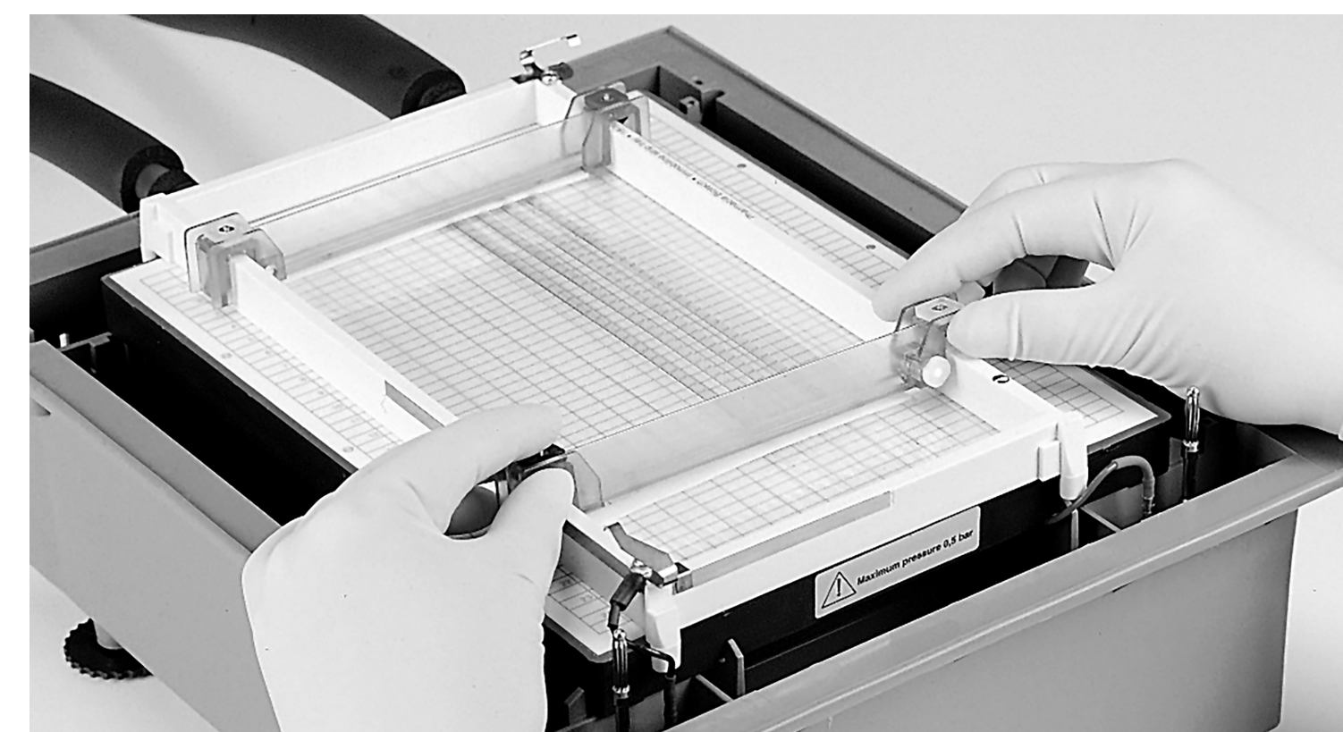
Fig 49. Alignment of electrodes over Immobiline DryStrip gels.
