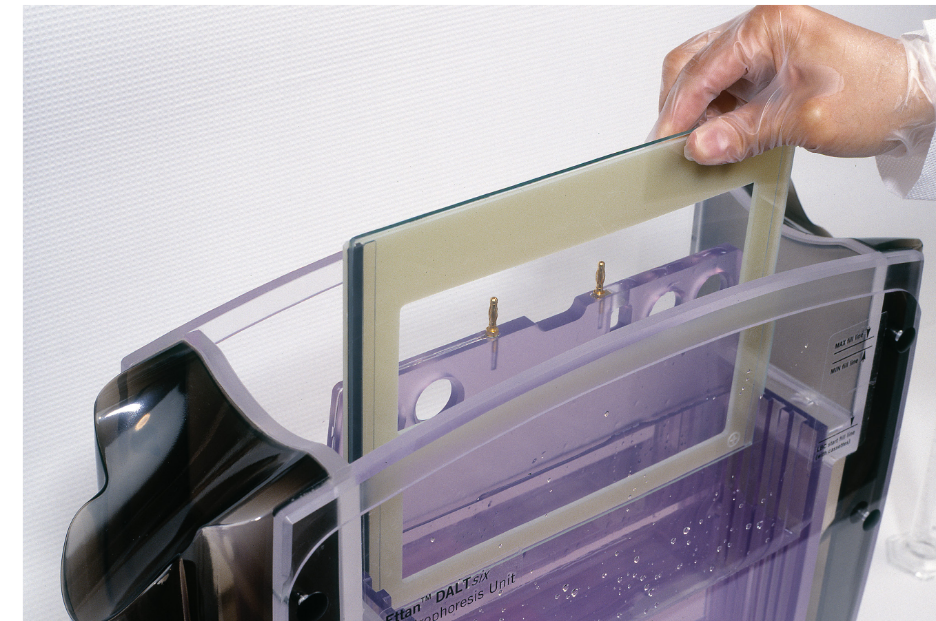
Fig 42. Inserting the cassettes into the cassette carrier.
