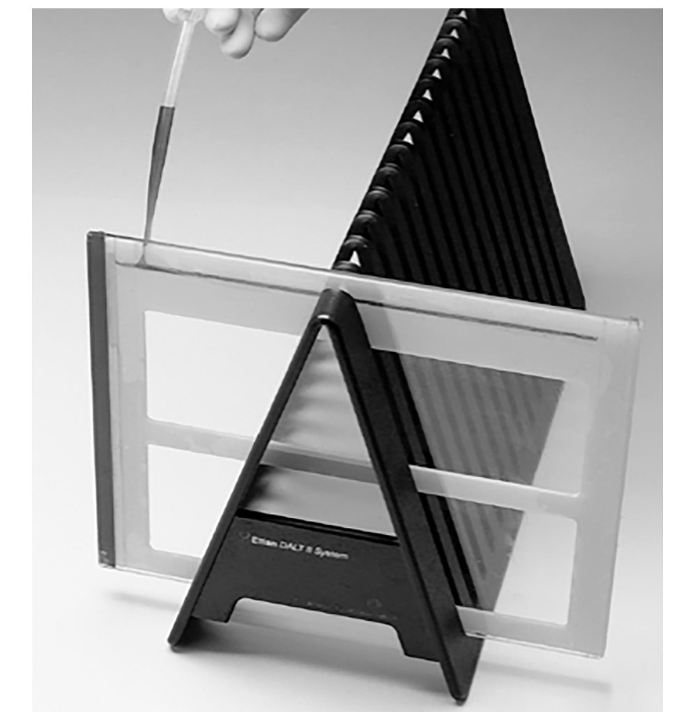
Fig 41. Sealing the Immobiline DryStrip gel in place on a DALT precast gel using agarose sealing solution.
