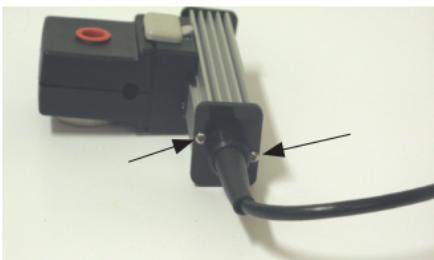
2. Slide the old lamp out of the lamp housing.
