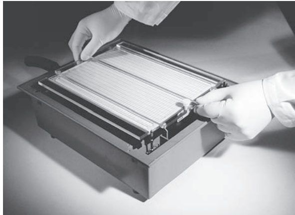
Figure 3.1: Placing the positioner over the gel and cooling plate
