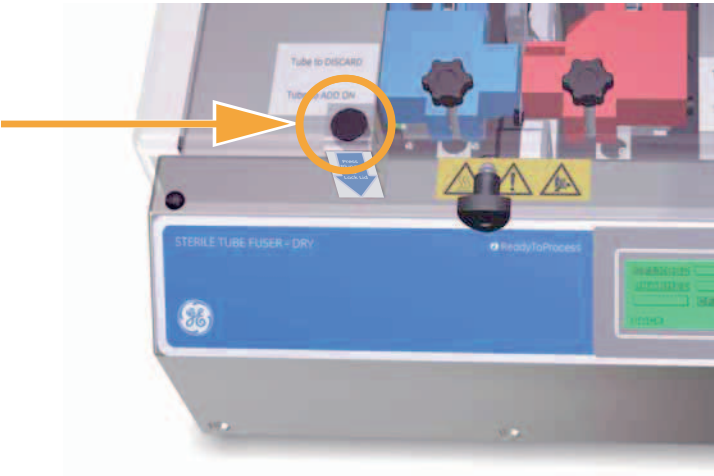
Fig 3-2. COVER LOCK button down — lid is locked.
