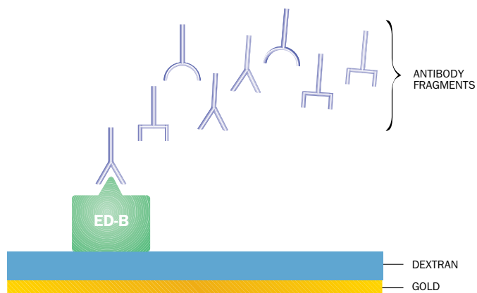
Fig 4. Biacore system was used to screen Ab fragment libraries to compare binding properties to ED-B immobilized on a Biacore sensor chip.
