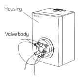
As the channel plate is turned by the motor, different ports are connected. Valve switching is controlled from UNICORN by reading the actual position of the channel plate.
