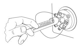
nplete Two techniques can be used for filling the sample loop filling.
