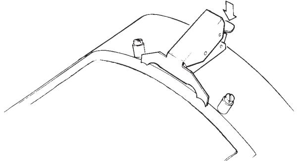
5 Pass the tension and wire over to the right handle so that the wire is now stretched over the gel-free part of the support film.
