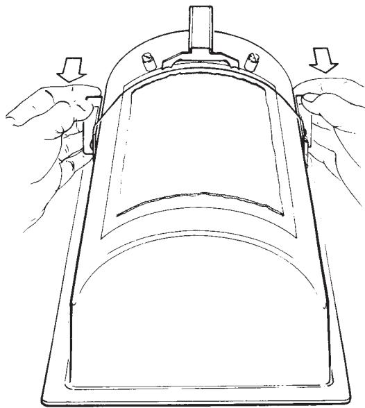
8 Release the tension lever and, without touching the upper surface of the gel, move the tension lever and wire over to the left side. Immediately clean the wire with a dry tissue as any residual gel will solidify and damage the lower surface of the next gel being separated.
