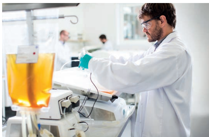
Fig 3. Quickly connect aseptically to downstream operations with Cellbag™ bioreactors that have ReadyMate™ connectors.
