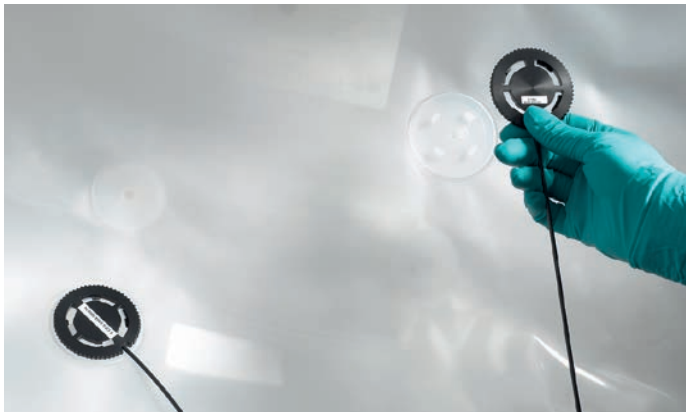
Fig 4. The optical sensor is embedded in the underside of the Cellbag™ bioreactor. Shown here is the bag adapter/optical fiber cable attached to the bag port.
